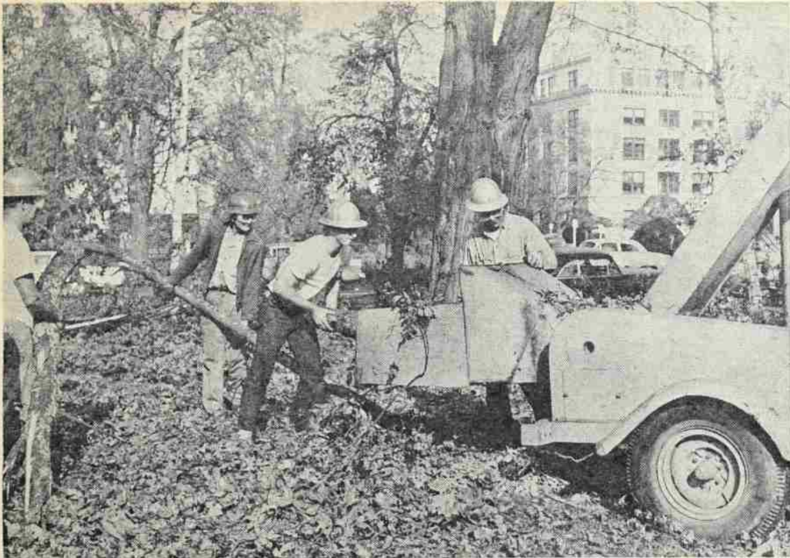
While Willamette students were busily grinding away at classes and assignments, workers hit the campus to grind the debris into chips of sawdust. The sawdust will be used for fuel at Fairview; so perhaps a very small good will come from Willamette's tragic tree loss. The grinding process began early Saturday morning and lasted through the week. (Photo by Burr Baughman).
