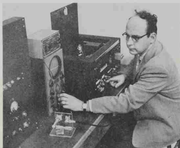
Dr. Robert Purbrick, Professor of Physics, at his Geiger counter in his laboratory. Dr. Purbrick built this extremely sensitive Geiger counter himself. Here he is testing a piece of fused sand from the first atomic test of 1945 in New Mexico. The Geiger counter was clicking madly at the time this picture was taken.
