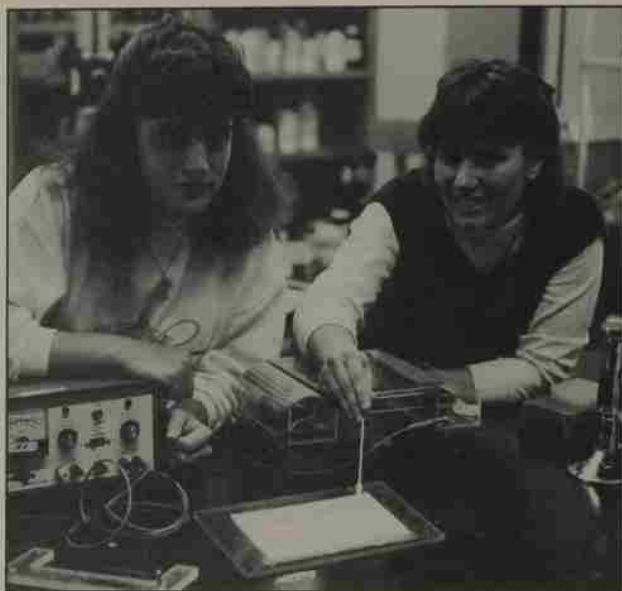
Susan Kephart (right) demonstrates the electrophoresis apparatus which she set up at Willamette during her sabbatical. It is for use by faculty and students conducting biochemical studies. Kephart is pointing to a gel, on which the dark bands represent proteins of different individuals, migrating in an electrical field. Darcie Flanagan (left) is a student who worked on research with her afterward. Flanagan's research was one of 14 projects funded by the new Undergraduate Research Grants program at Willamette.
