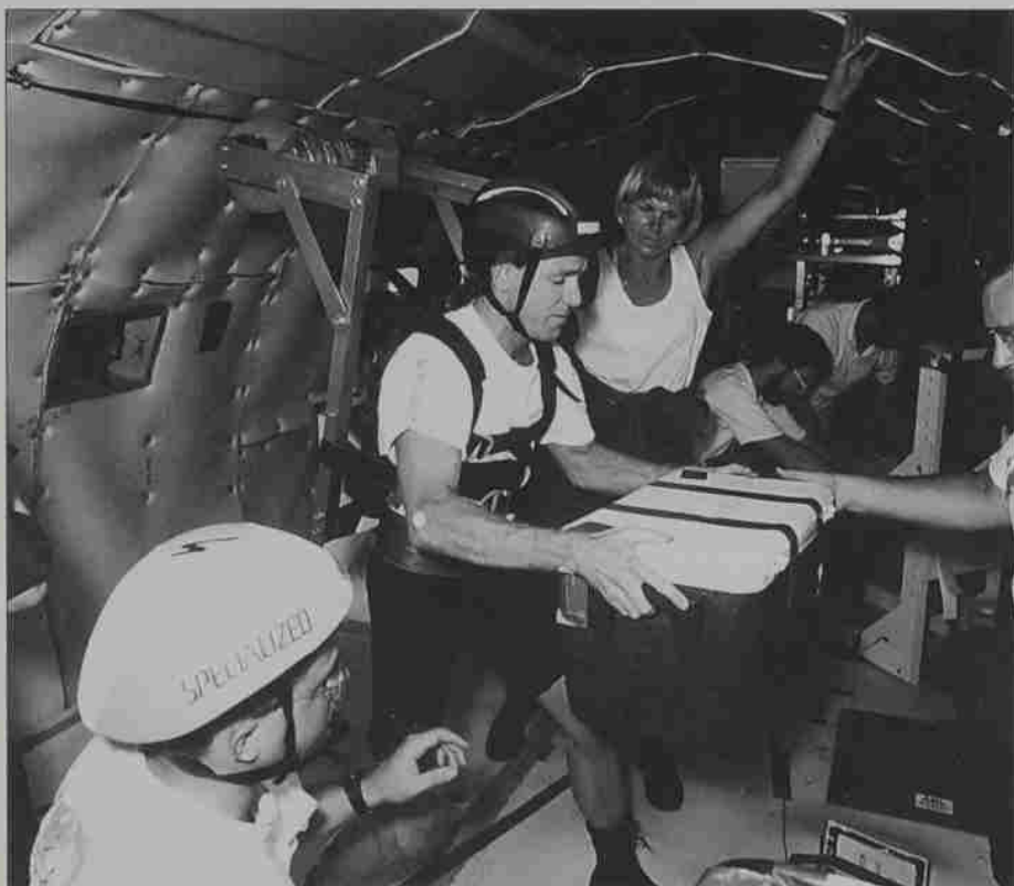
Leslie Wickman is shown on board a KC135 research aircraft which uses centripetal acceleration to cancel out gravity. The objective of the tests being conducted is to determine, with the use of weighted backpacks, the most efficient load distribution for different gravities, in this case Martian and lunar gravities.
